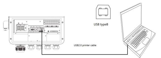
The user can read and modify device parameters through this port by using the host software. Please contact us for the host software installation package if you require one.
